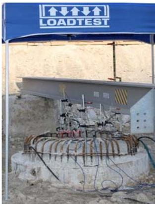
Pile head test arrangement showing reference beam during O-cell bi-directional loading in progress.
